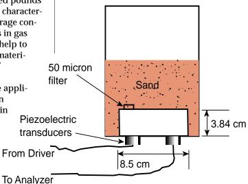
Gas resonance modes are identified by comparing spectra acquired with the container under vacuum and filled with argon at a pressure of 40 psia. All observed gas resonances match with calculated resonances. Gas amplitudes are typically quite small, about one-tenth the amplitude of the continuous background and one-hundredth the amplitude of the strongest container mode observed.
